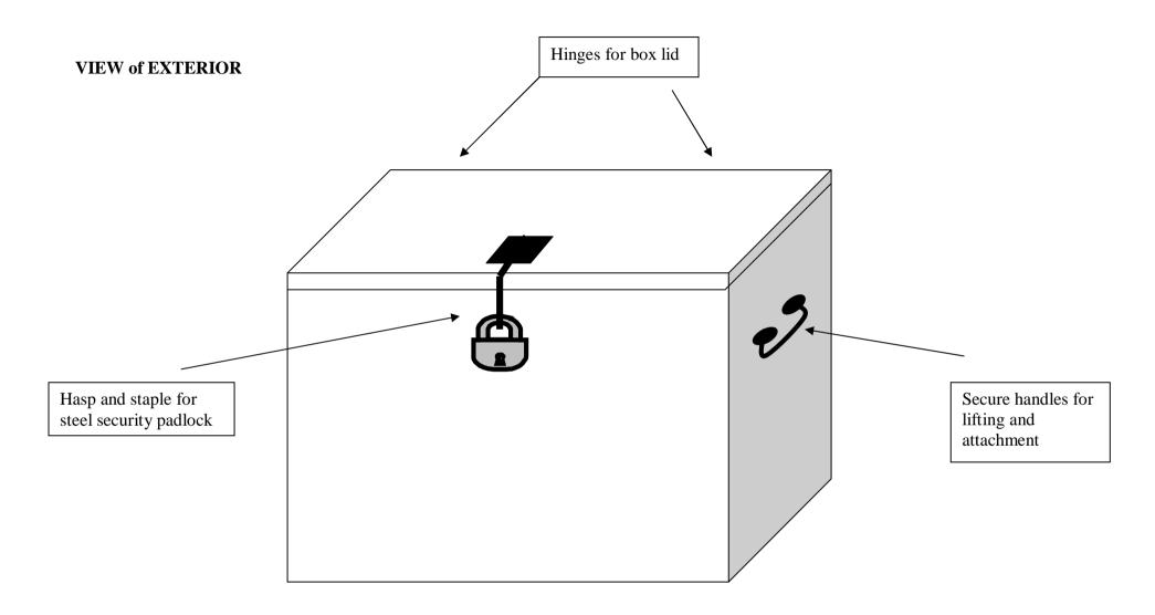
NOTE: Screws for handles, hasp & staple and hinges not to penetrate to inside of box
